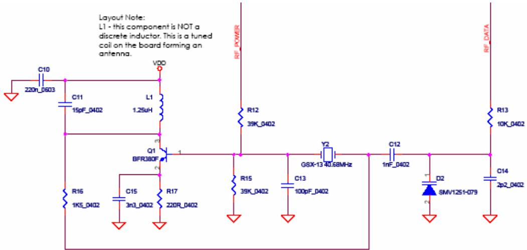
Transmitter Circuit Diagram (excluding PIC data driver)
