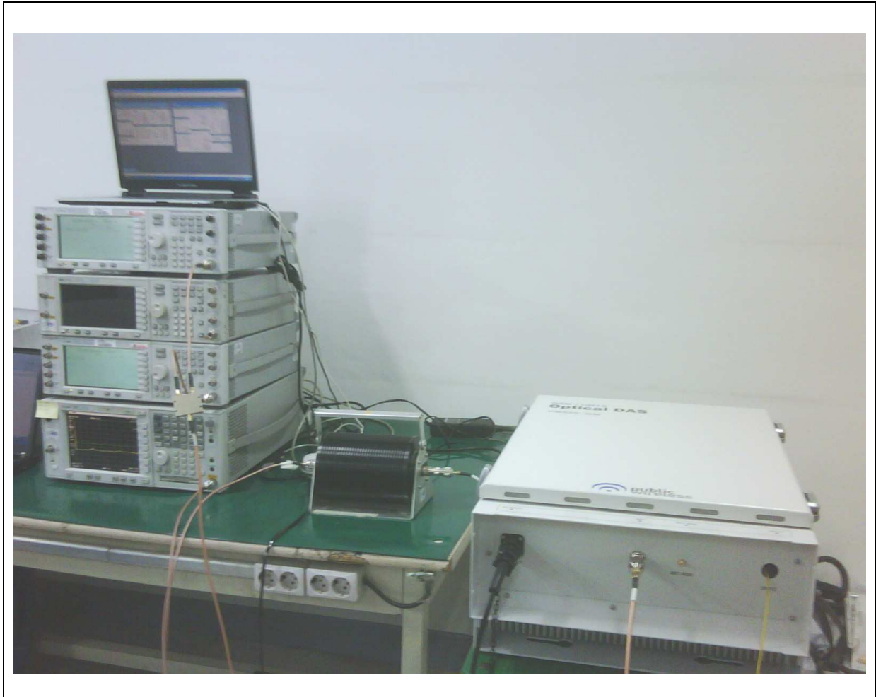
Figure 4 Test setup for Conducted Measurement
