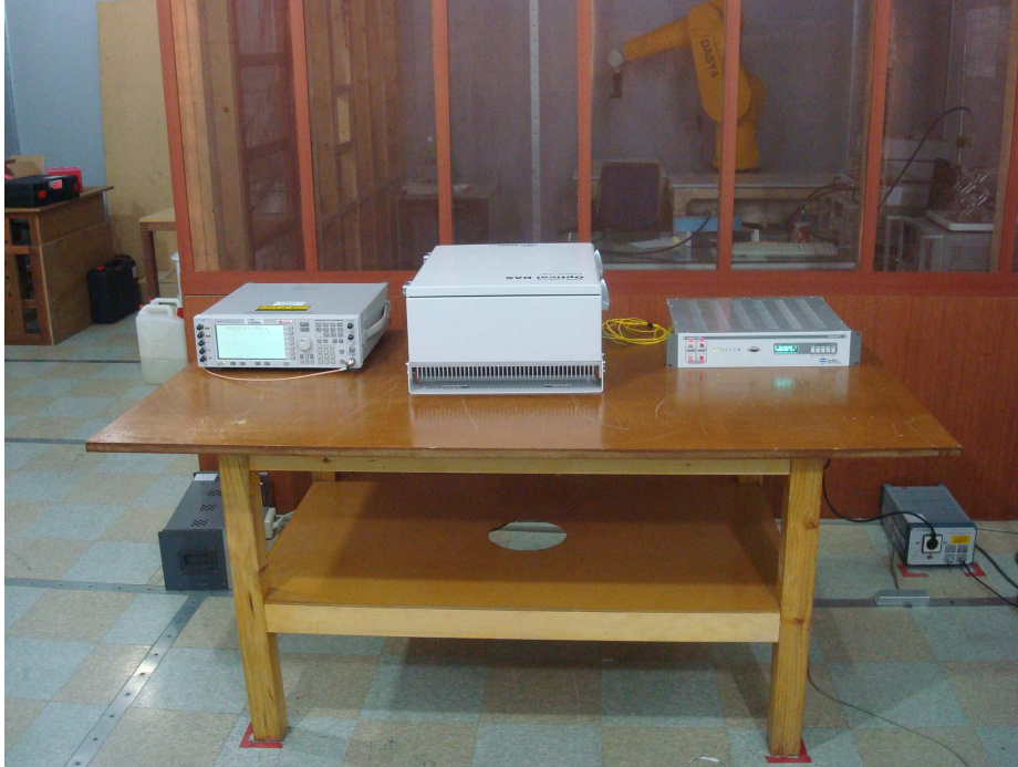
Figure 1 Test Setup for Conducted Emissions
