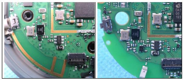
2.DECT antenna change: Antenna position and material change, SAR and radiation spurious have been retested.
