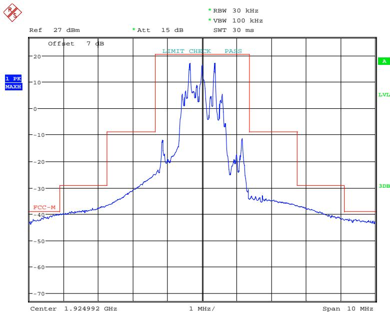
**High Channel (Unwanted Emission inside the Sub-band)**
