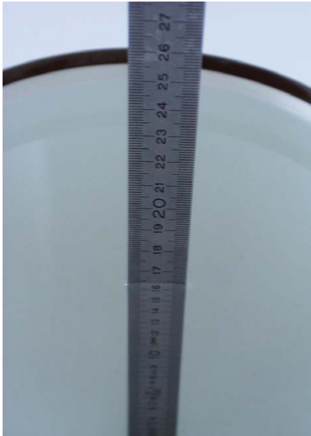
Fig. 23: Liquid depth for 1900 MHz Head measurements
