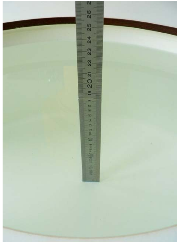
Fig. 24: Liquid depth for 1900 Body worn measurements
