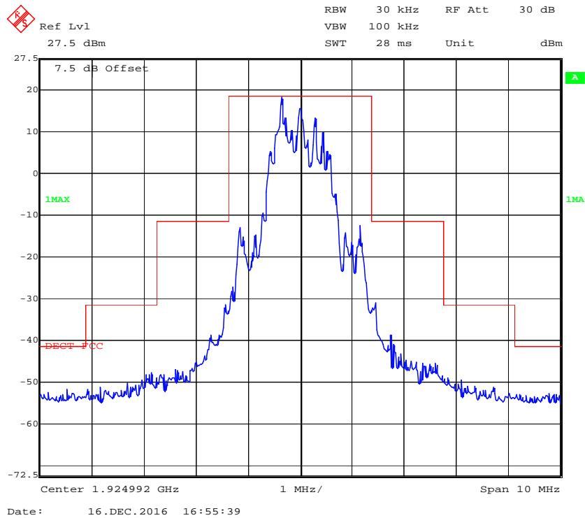
**High Channel (Unwanted Emission inside the Sub-band)**
