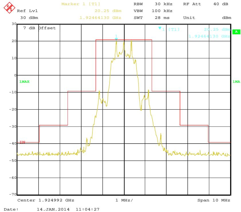
**High Channel (Unwanted Emission inside the Sub-band)**
