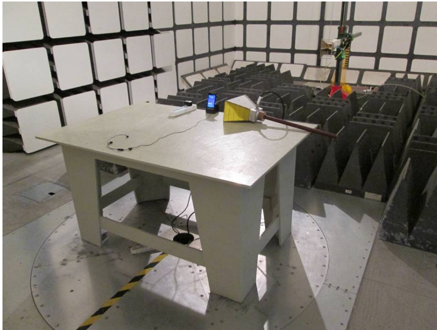
Radiated Emissions – Front View (1-25 GHz)
