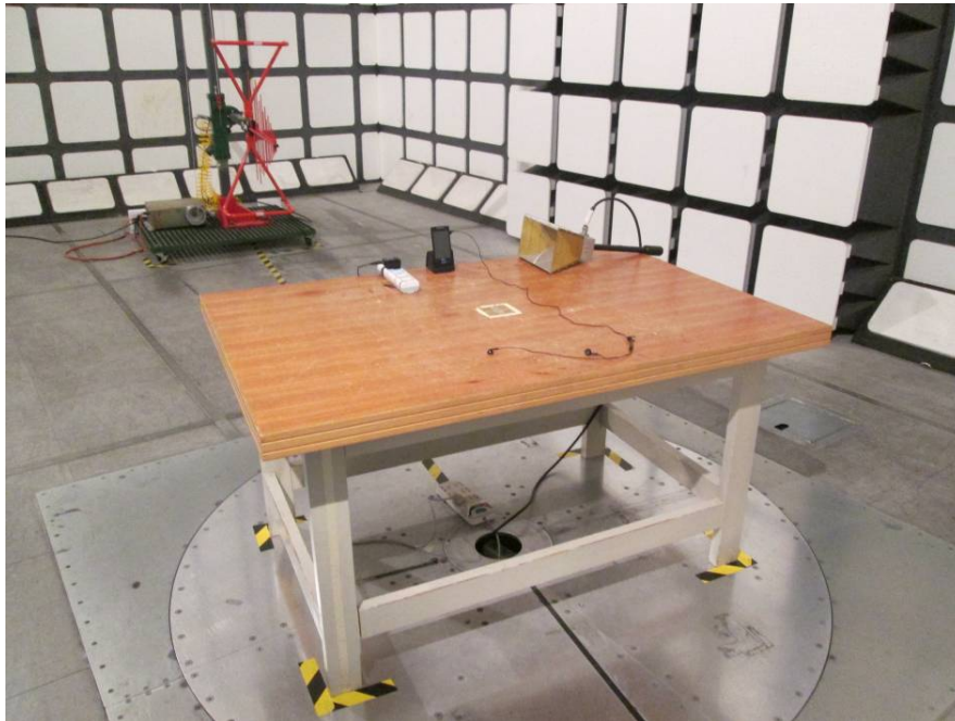
Radiated Emissions – Front View (30-1000 MHz)
