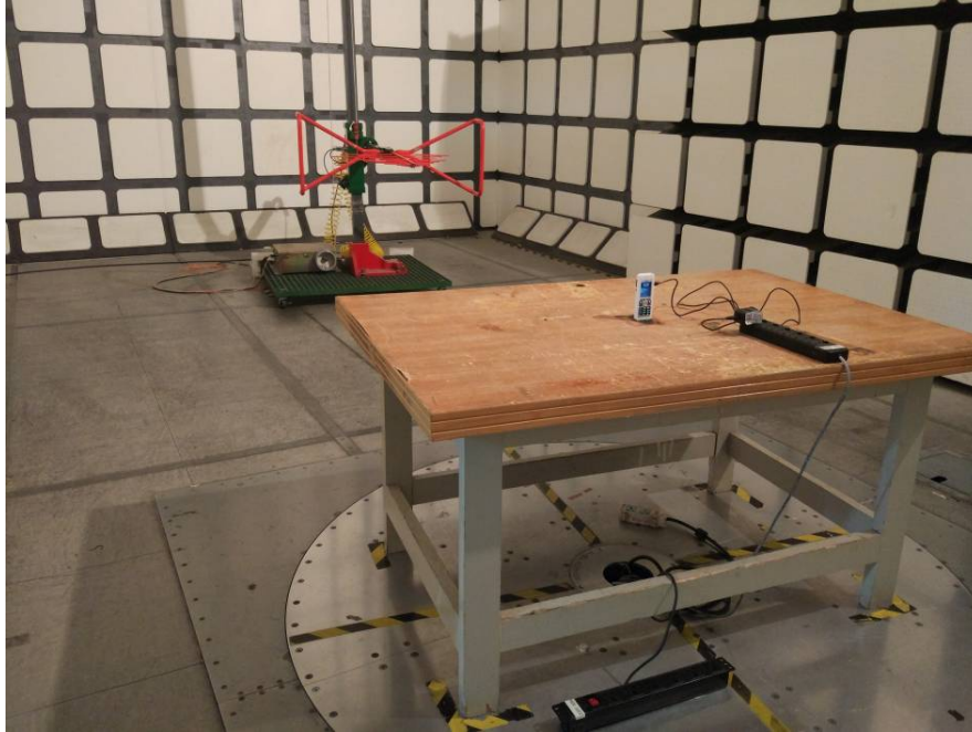
Radiated Emissions View (Below 1 GHz, Charging by Adapter)
