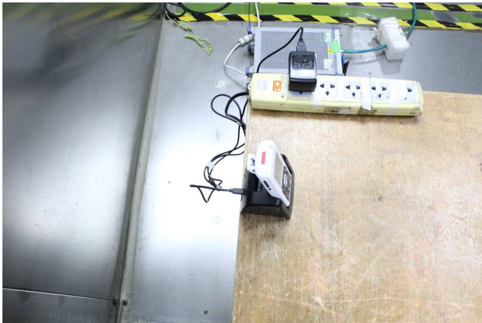
Conducted Emissions - Side View (Charging by Charger 1)
