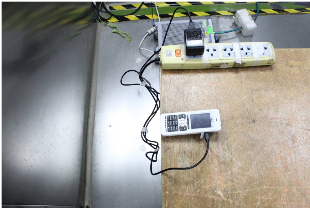
Conducted Emissions - Side View (Charging by Adapter)
