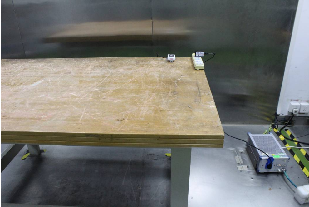
Conducted Emissions - Front View (Charging by Adapter)
