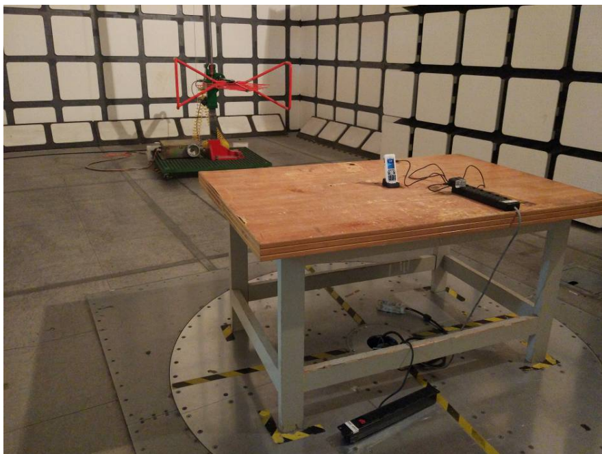
Radiated Emissions View (Below 1 GHz, Charging by Charger 2)
