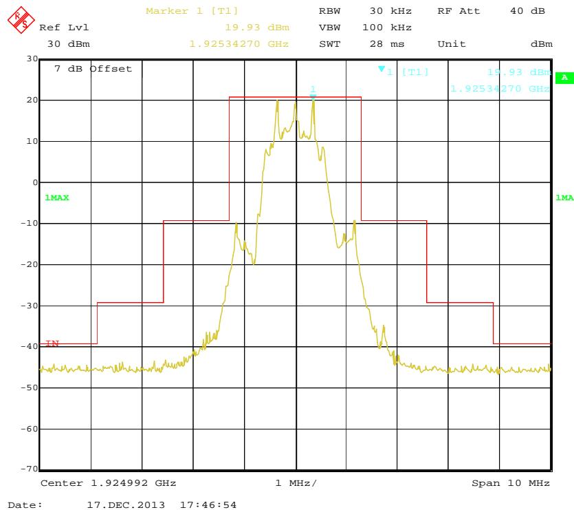
**High Channel (Unwanted Emission inside the Sub-band)**
