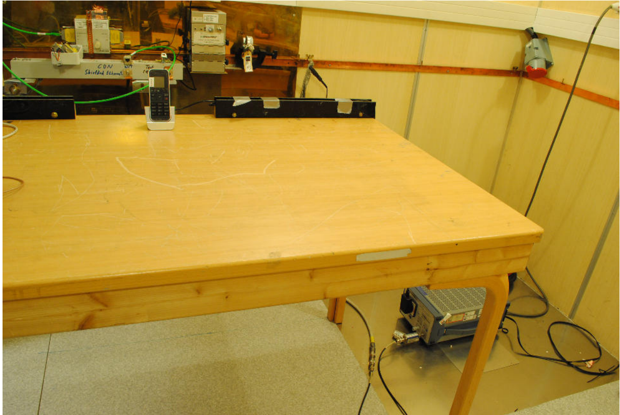
Power line Conducted Emissions Test Set-up
