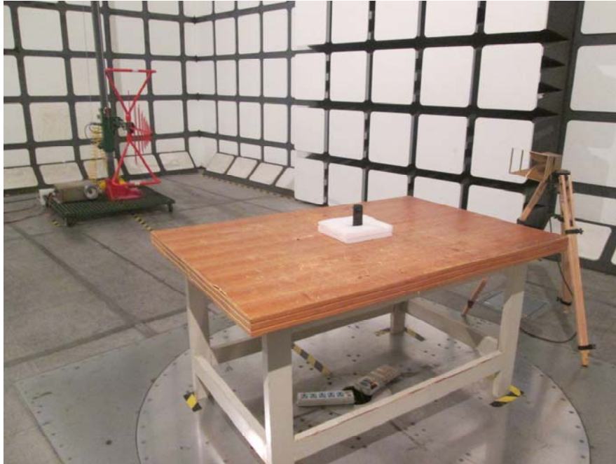
Radiated Emissions View (Below 1 GHz)
