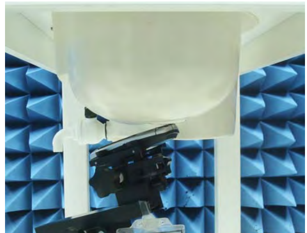
Figure 17. Left Head SAR Test Setup (Tilted)
