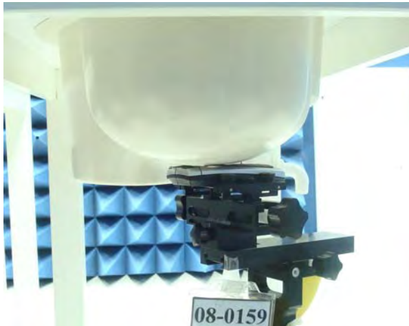
Figure 14. Right Head SAR Test Setup (Cheek)
