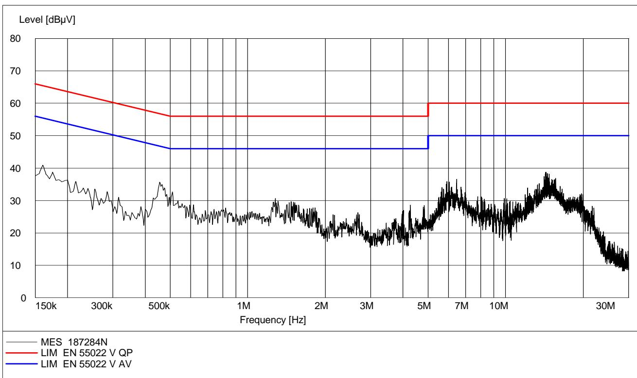
**Handset Charging, Phase L1 and N, 120V 60Hz (plot shows worst case of the two phases)**
