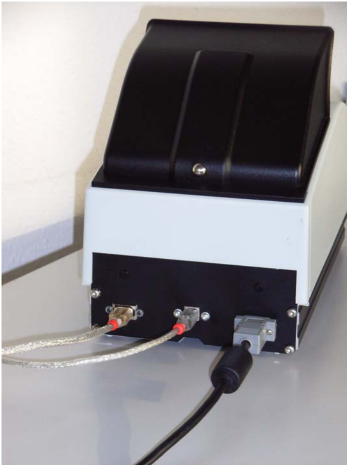
Figure 5: ID-Star 4054 ePR with power supply and attached interface cables.
