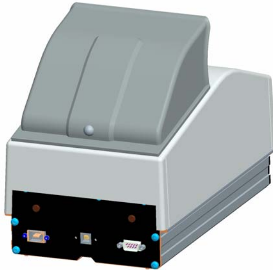
Figure 4: Connections on the ID-Star 4054 ePassport Reader
