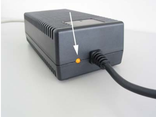
Figure 8: Status LED on the power supply
