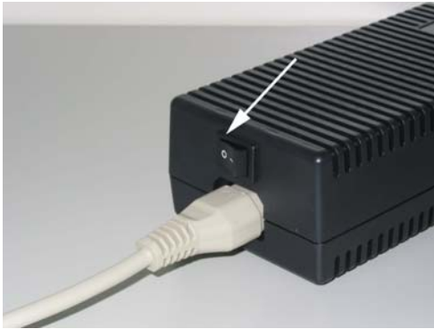
Figure 11: Switch in the 'OFF' position
