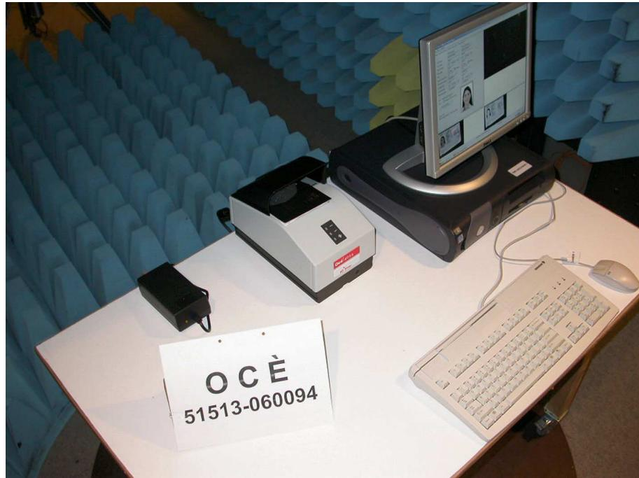
**Test setup for radiated emission measurement
