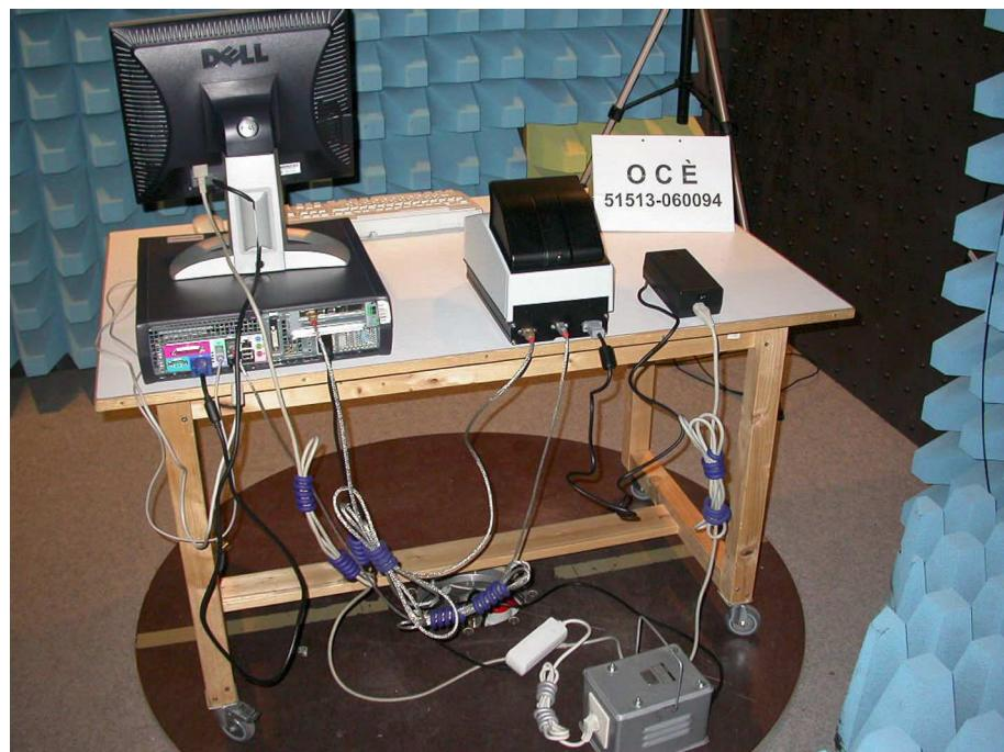
**Test setup for radiated emission measurement
