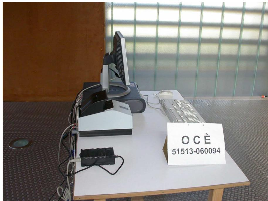
**Test setup for radiated emission measurement
