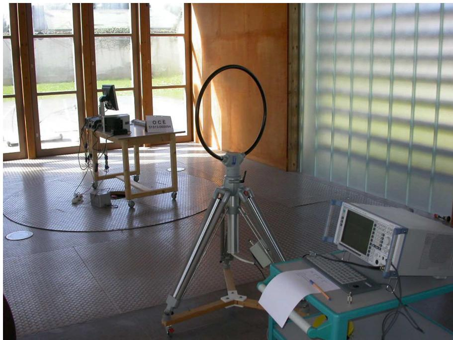
**Test setup for radiated emission measurement
