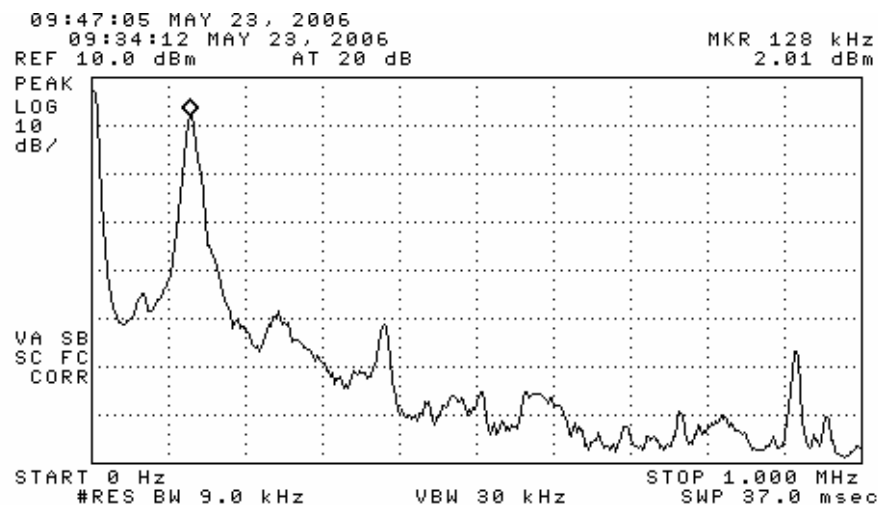
Figure 6.2. Emission spectrum of the DUT. The amplitudes are only indicative (not calibrated).
