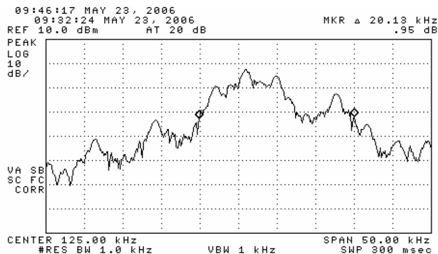
Figure 6.3. Measured bandwidth of the DUT. (pulsed)
