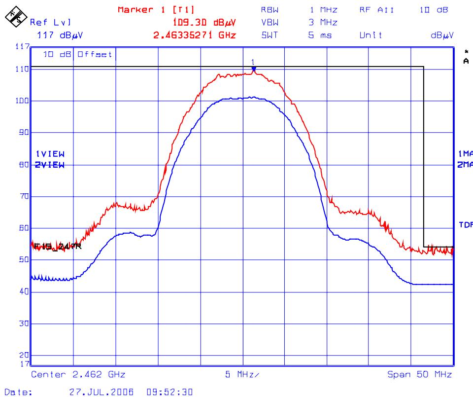
**Photo #6: Upper Band-Edge Radiated Emissions – Vertical Polarization**
