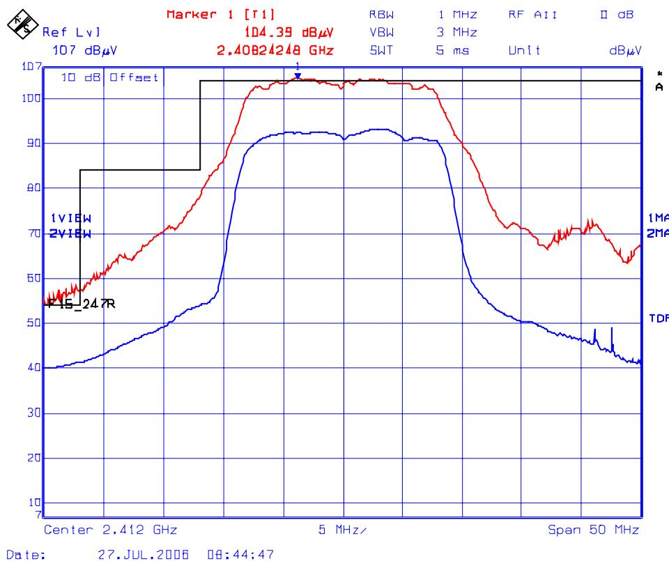
**Photo #12: Lower Band-Edge Radiated Emissions - Vertical Polarization**
