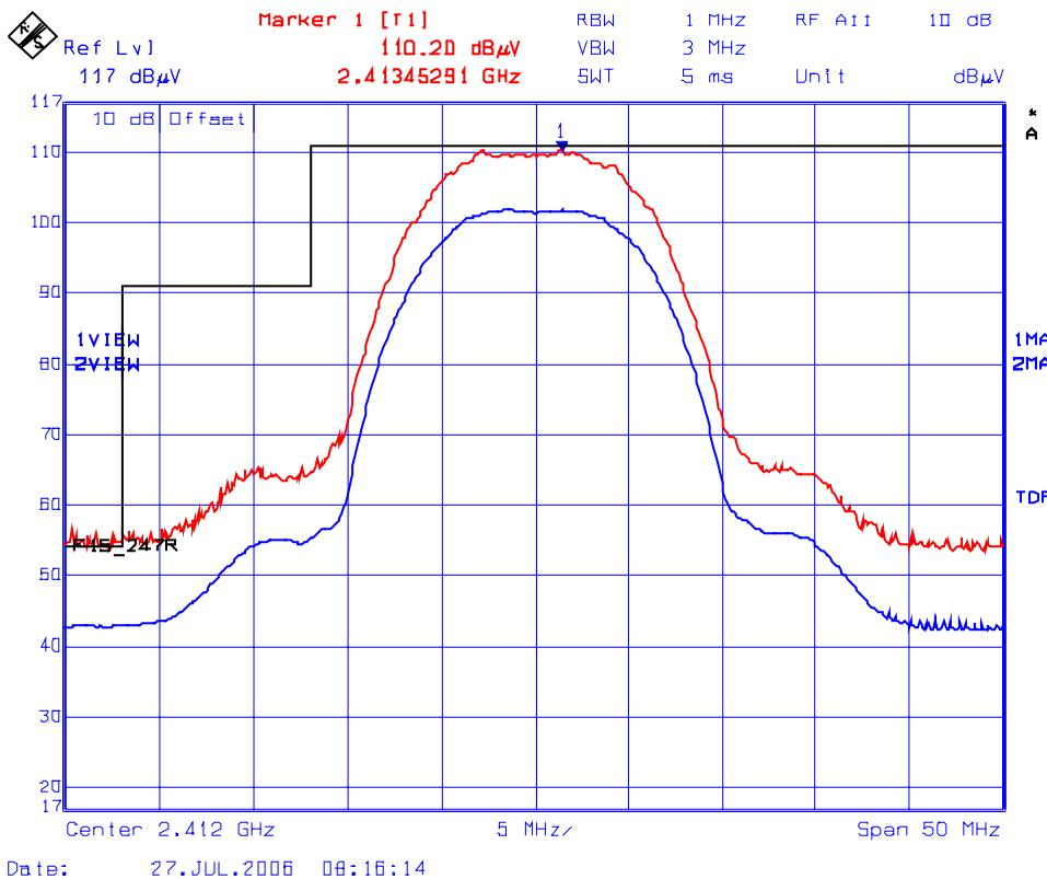
**Photo #5: Upper Band-Edge Radiated Emissions – Horizontal Polarization**
