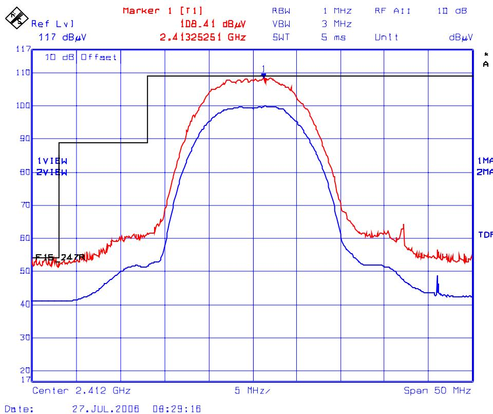
**Photo #4: Lower Band-Edge Radiated Emissions – Vertical Polarization**
