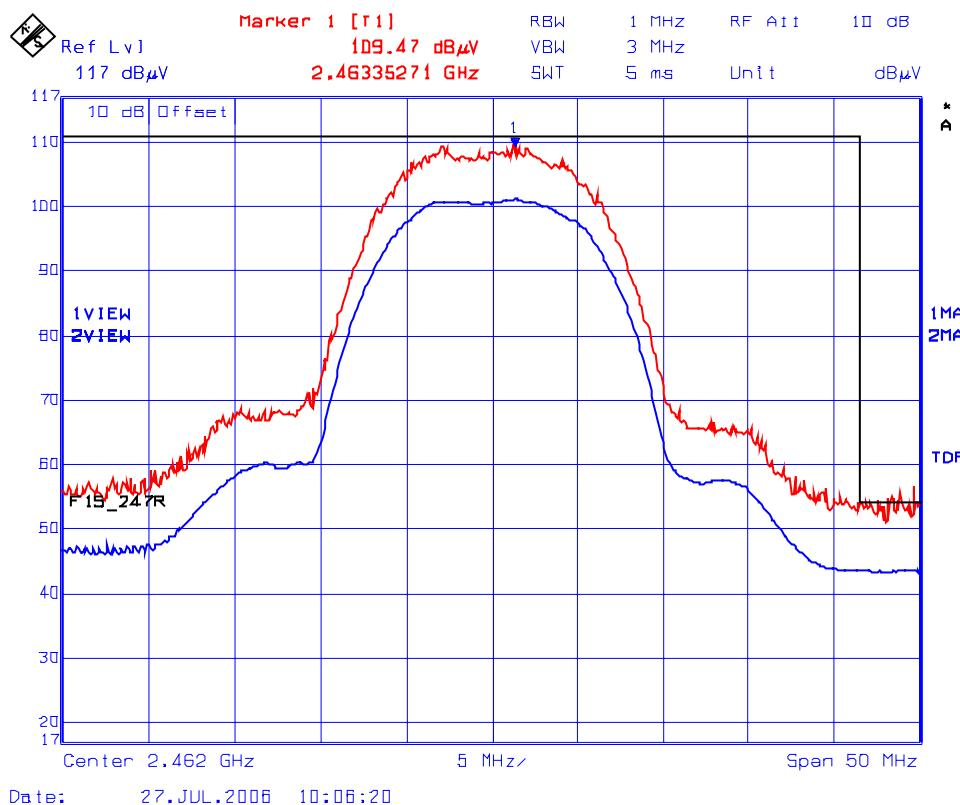
**Photo #7: Lower Band-Edge Radiated Emissions - Horizontal Polarization**
