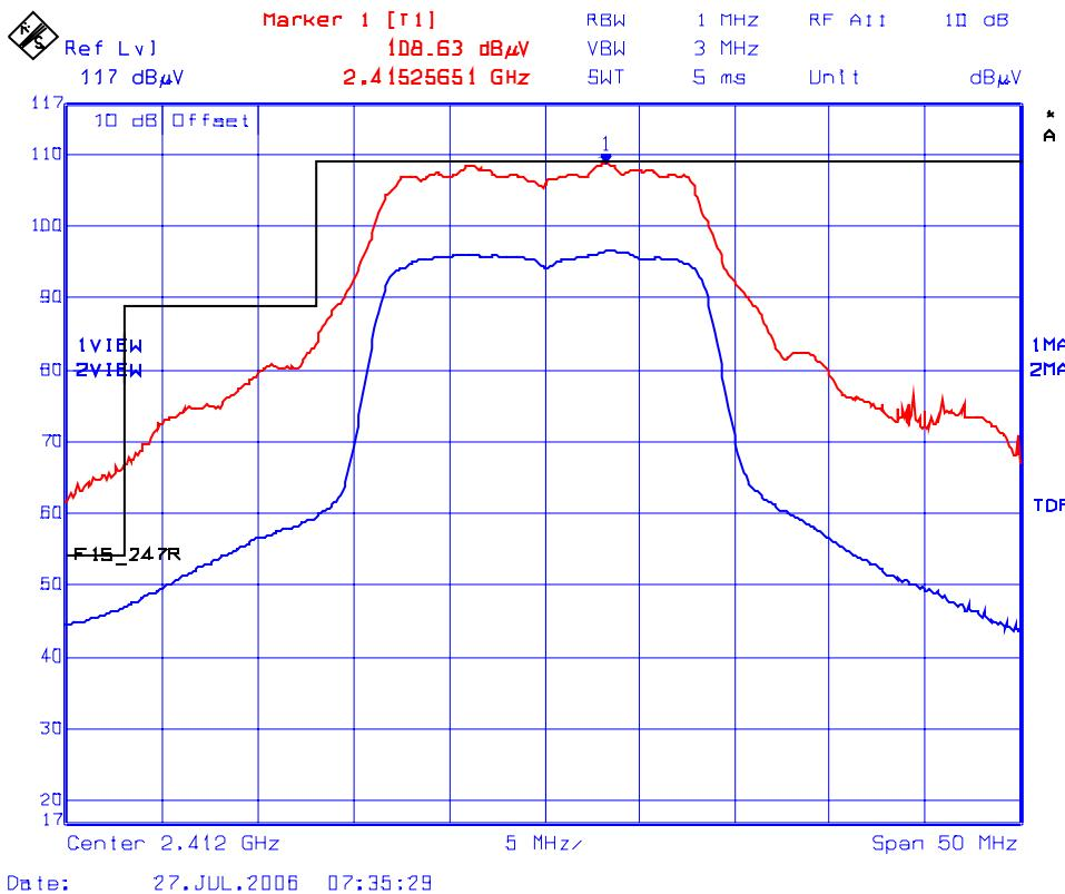
**Photo #13: Upper Band-Edge Radiated Emissions - Horizontal Polarization**
