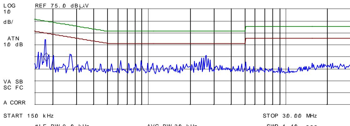
**Plot #2: AC POWER LINE CONDUCTED EMISSIONS MEASUREMENT PLOT**
