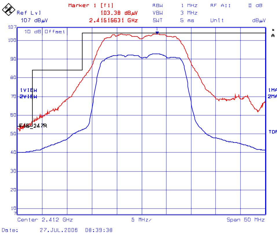
**Photo #8: Lower Band-Edge Radiated Emissions - Vertical Polarization**
