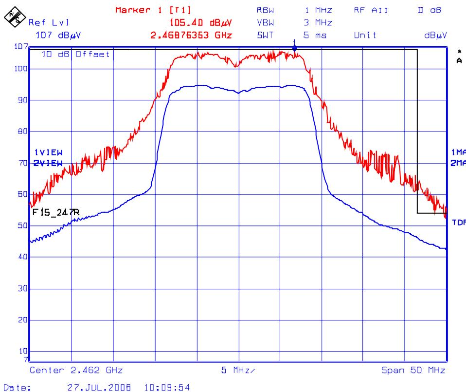
**Photo #11: Lower Band-Edge Radiated Emissions - Horizontal Polarization**
