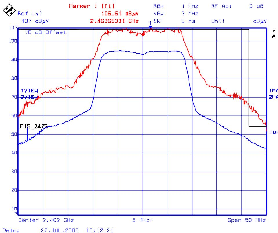
**5.12.5.2. Transmitter Radiated Spurious Emissions**
