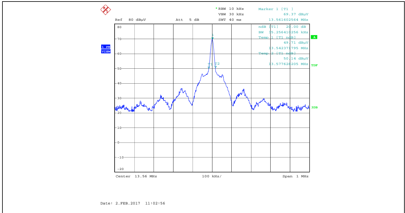
Plot 5.2.3.5. 20 dB Bandwidth, Fc: 13.56 MHz, Technology B, Bit Rate 106
