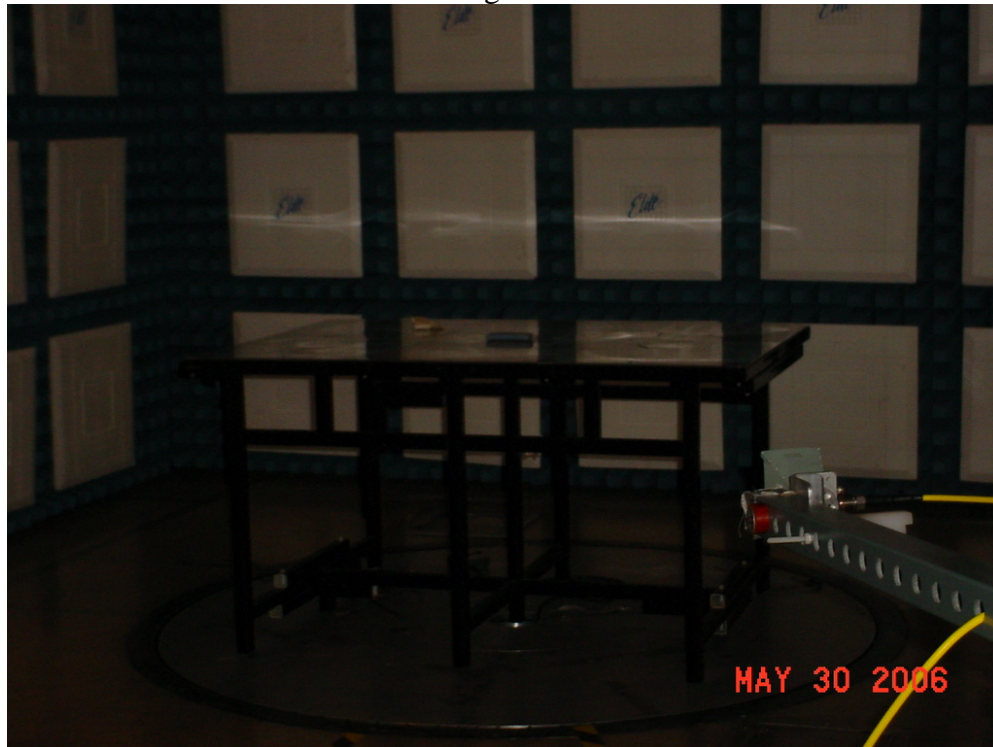
Test Setup for Radiated Emissions – Horizontal Polarization
