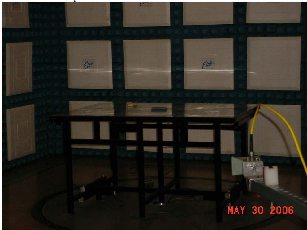
Test Setup for Radiated Emissions – Vertical Polarization
