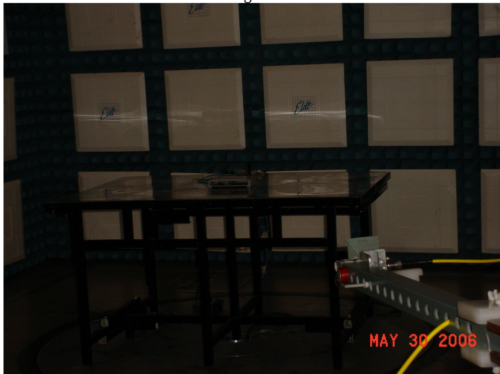
Test Setup for Radiated Emissions – Horizontal Polarization
