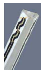
Figure 3.2 Probe Thick-Film Technique
