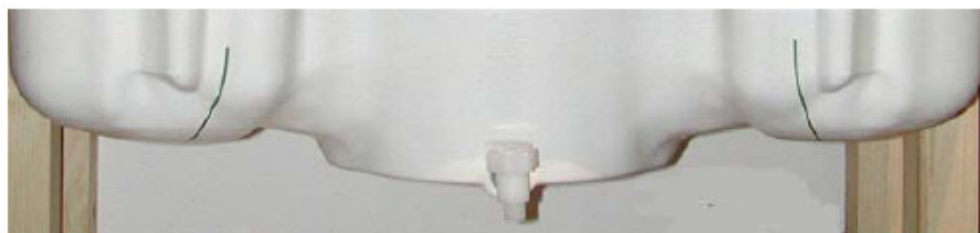
Figure 7.2 SAM Twin Phantom shell
