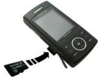
When you need to remove the T-Flash card, you should switch off the phone before removing the T-Flash card from right side of the phone.
