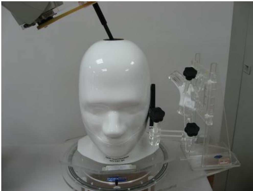
Fig.3 EUT Left Head Touch Cheek Position
