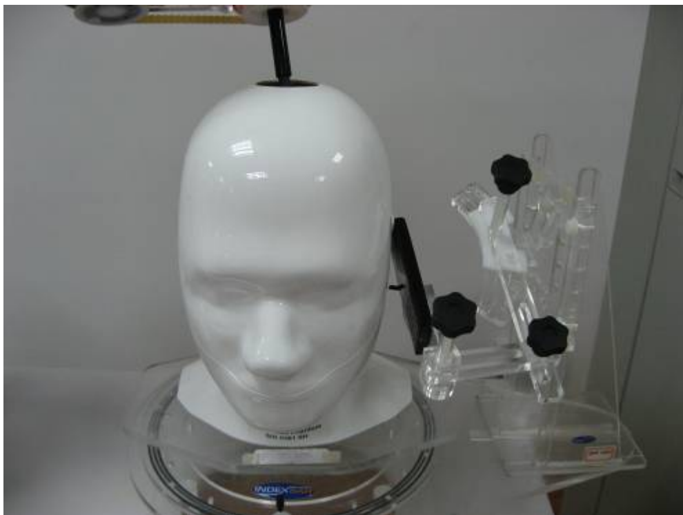
Fig.4 EUT Left Head Tilt15 Position
