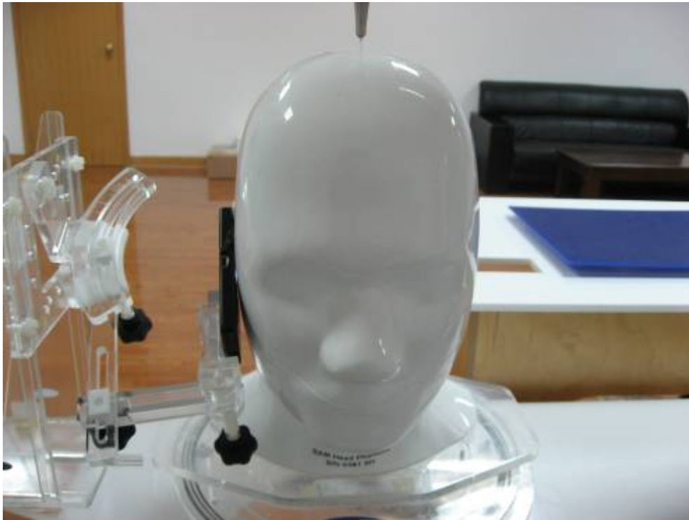
Fig.5 EUT Right Head Touch Cheek Position
