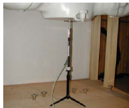
Figure 12.1 Dipole Validation Test Setup
