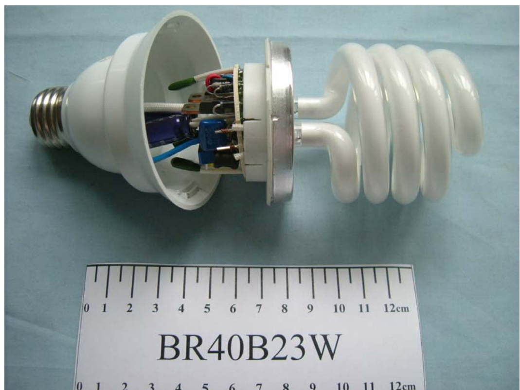
FIGURE 2 SELF-BALLASTED LAMP (M/N: BR40B23W) TUBE REMOVED
