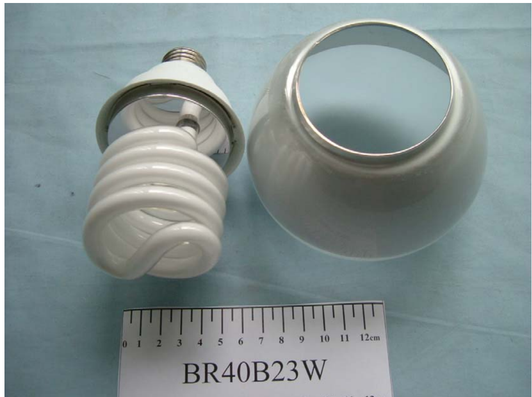
FIGURE 1 SELF-BALLASTED LAMP (M/N: BR40B23W) LAMP SHADE REMOVED
