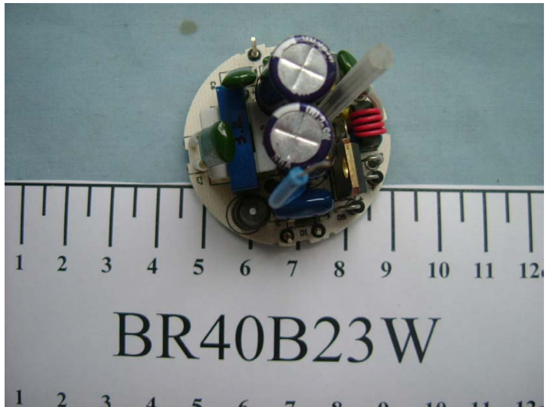
FIGURE 3 SELF-BALLASTED LAMP (M/N: BR40B23W) MAIN BOARD (COMPONENT SIDE)
