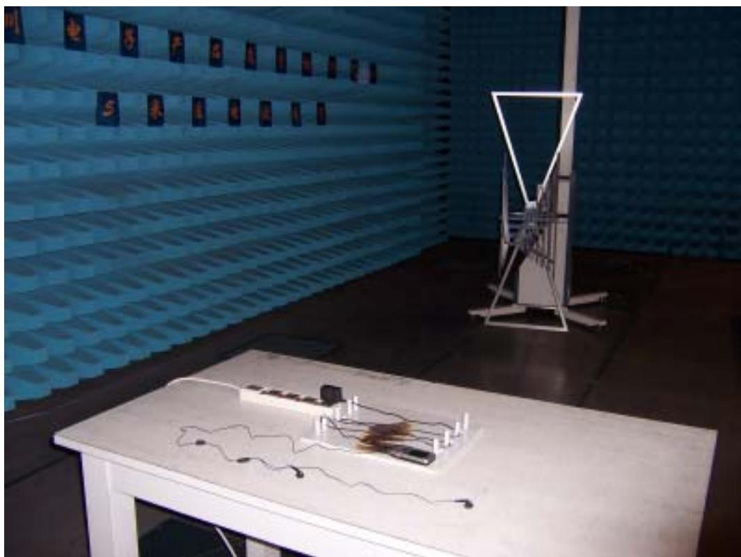
**4. Radiated Emission Test, USB Mode**
