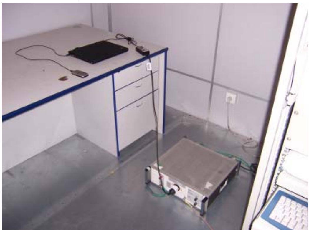
**3. Radiated Emission Test, Charging Mode**
