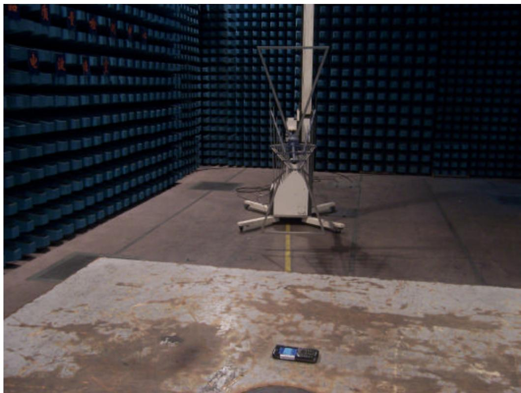
**4. Radiated Emission Test (above 1 GHz)**
