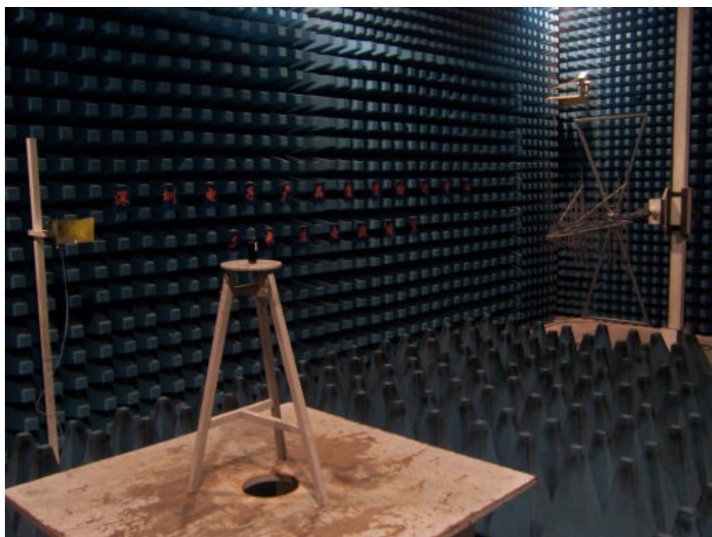
**3. Radiated RF Test (9kHz~30MHz)**
