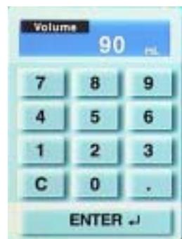
Injection volume is set with the numerical key pad.
