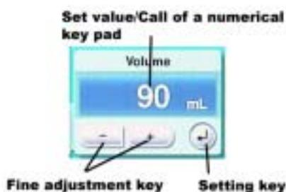
Touch the frame of the injection volume. A fine adjustment key is displayed. Touch the frame of the set value. A numerical key pad will be displayed. A fine adjustment key disappears automatically in about five seconds.
