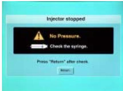
A low-pressure warning may be displayed and operation may be stopped, if pressure is not loaded continuously while 5 mL of drug solution is injected. Syringe, needle and injection route should be checked.
