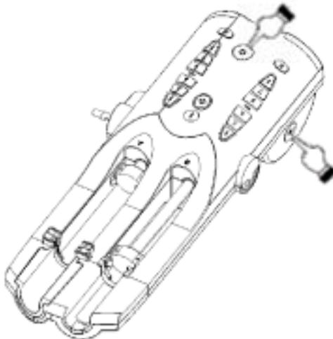
There are injection stop buttons on both sides and the top of the head.
