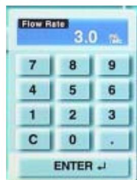
Injection flow rate is set with the numerical key pad.
