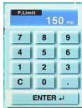
Touch the frame of the P.Limit (Pressure Limit). The numerical key pad will be displayed.
