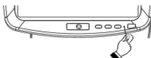
Push a switch in the inside of the hole with an end-rounded stick.
