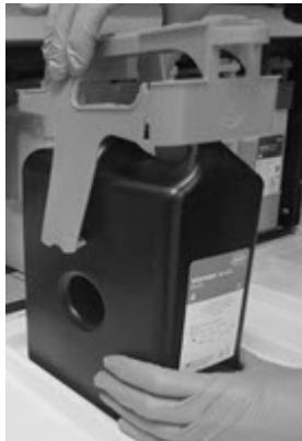
2 Wash the reagent hat and tubing with deionized water. Allow to dry.
