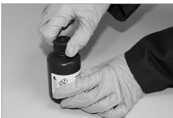
3 Remove the cap from the new coverslip activator bottle.
