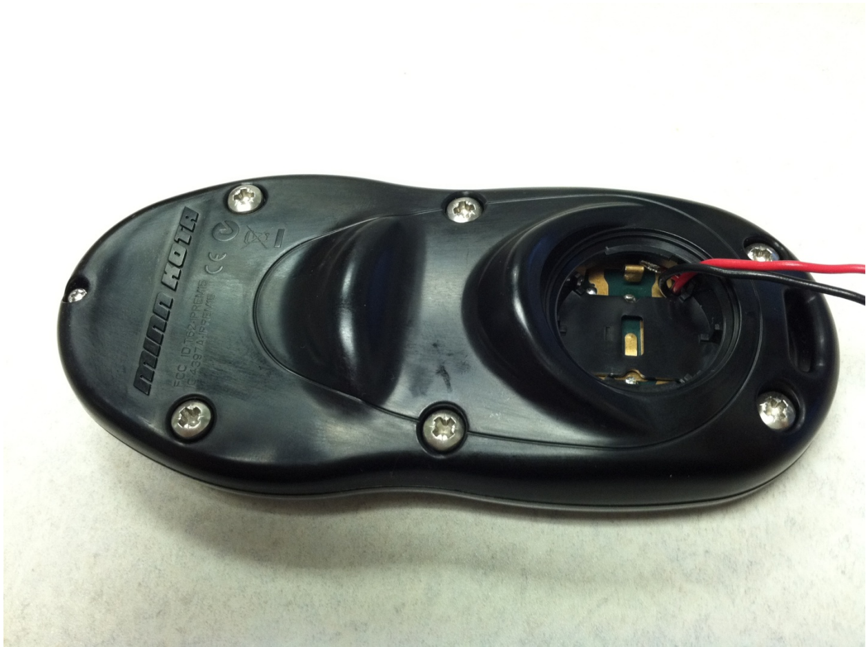
Figure 3 - Back of EUT showing location of screw near antenna
