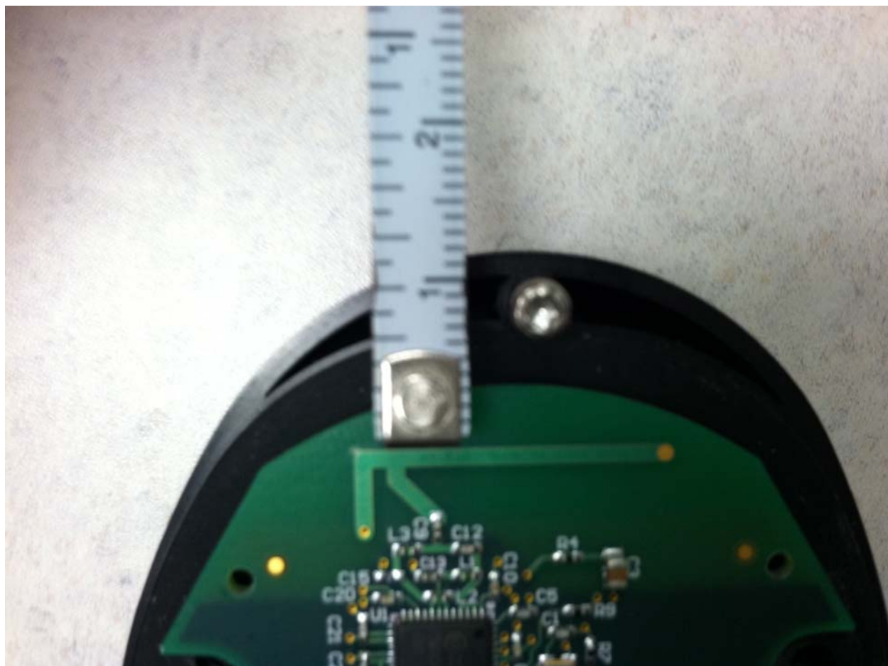
Figure 4 - Location of screw next to antenna (Measurements shown in centimeters)
