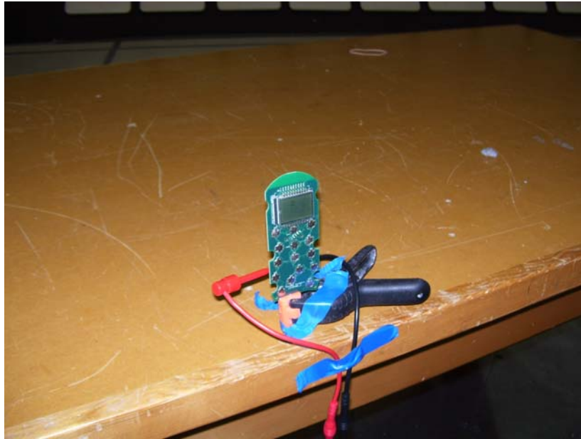
Figure 3 - Radiated Emissions Testing, 1 - 26GHz, Horizontal
