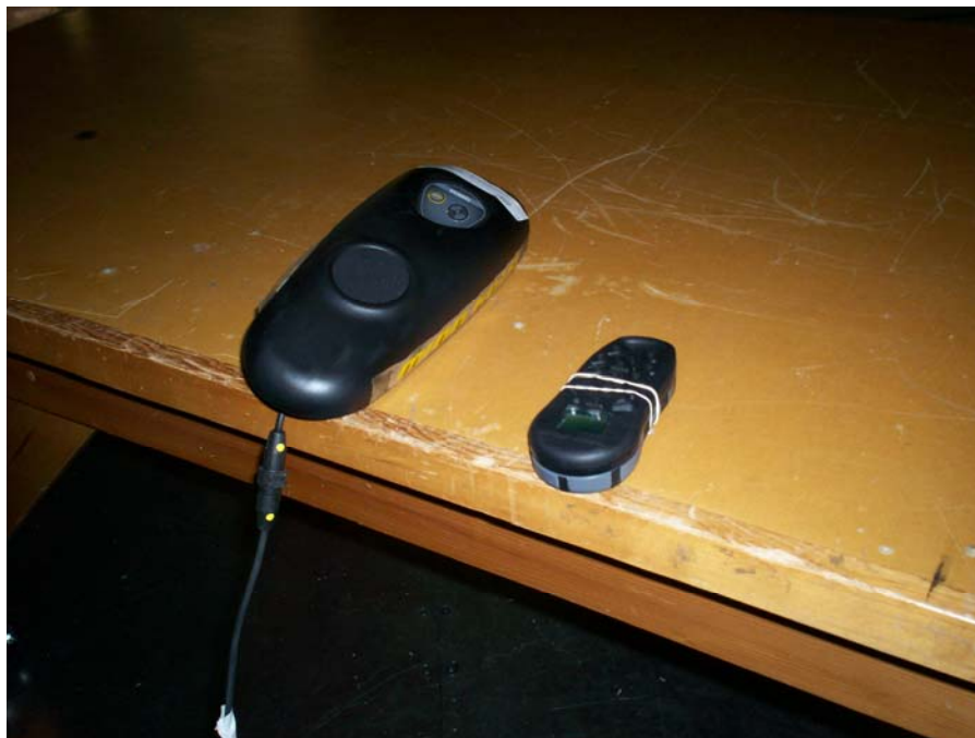
Figure 2 - Radiated Emissions Testing, 30MHz – 1GHz, Tested with i-Pilot Controller
