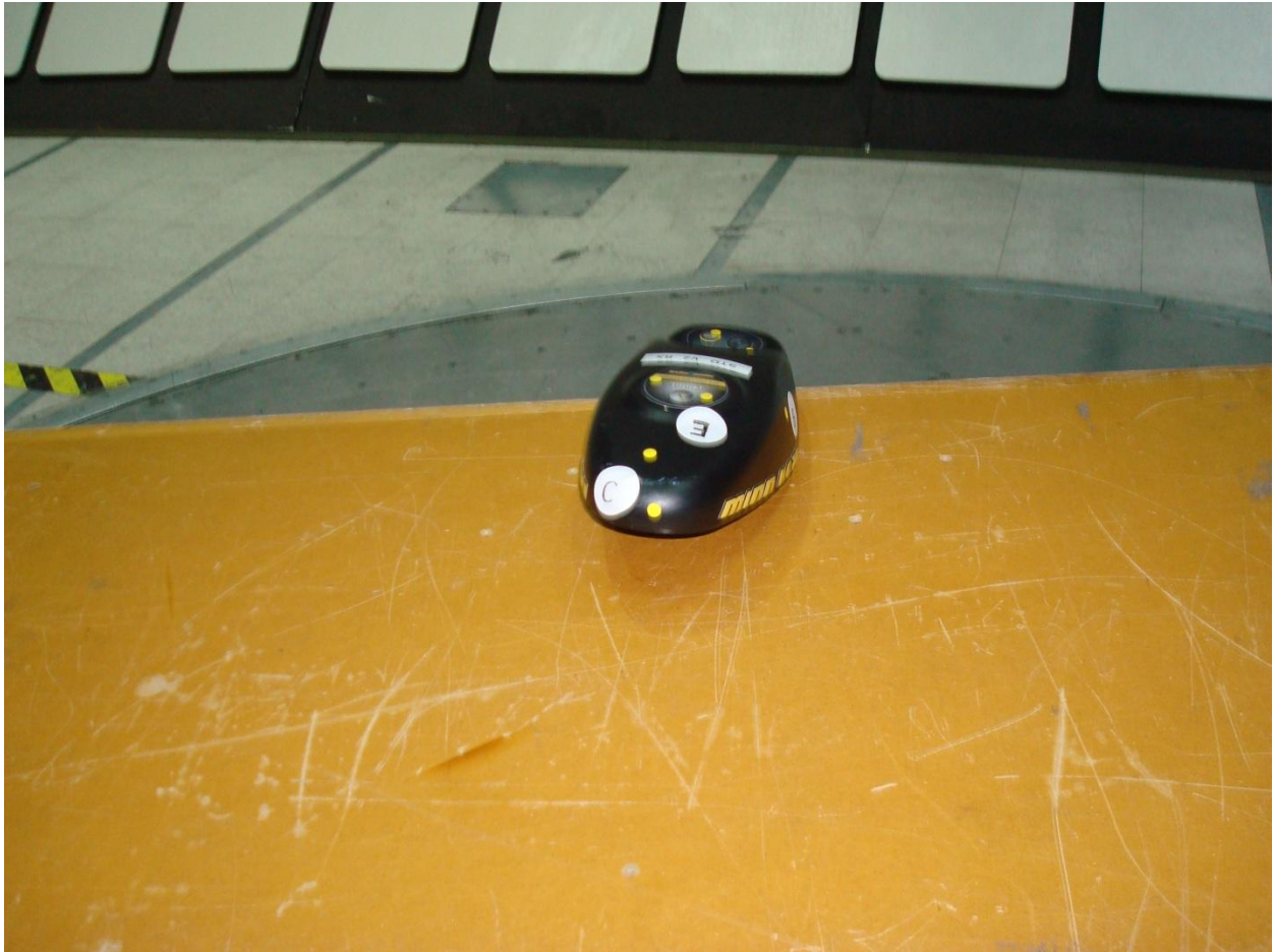
Figure 2 - i-Pilot Motor Controller Test Setup, Radiated Emissions
