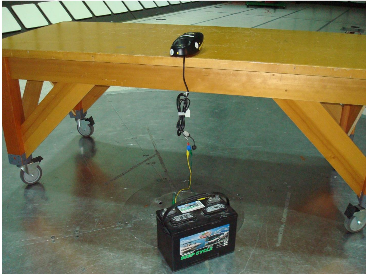
Figure 1 - i-Pilot Motor Controller Test Setup, Radiated Emissions
