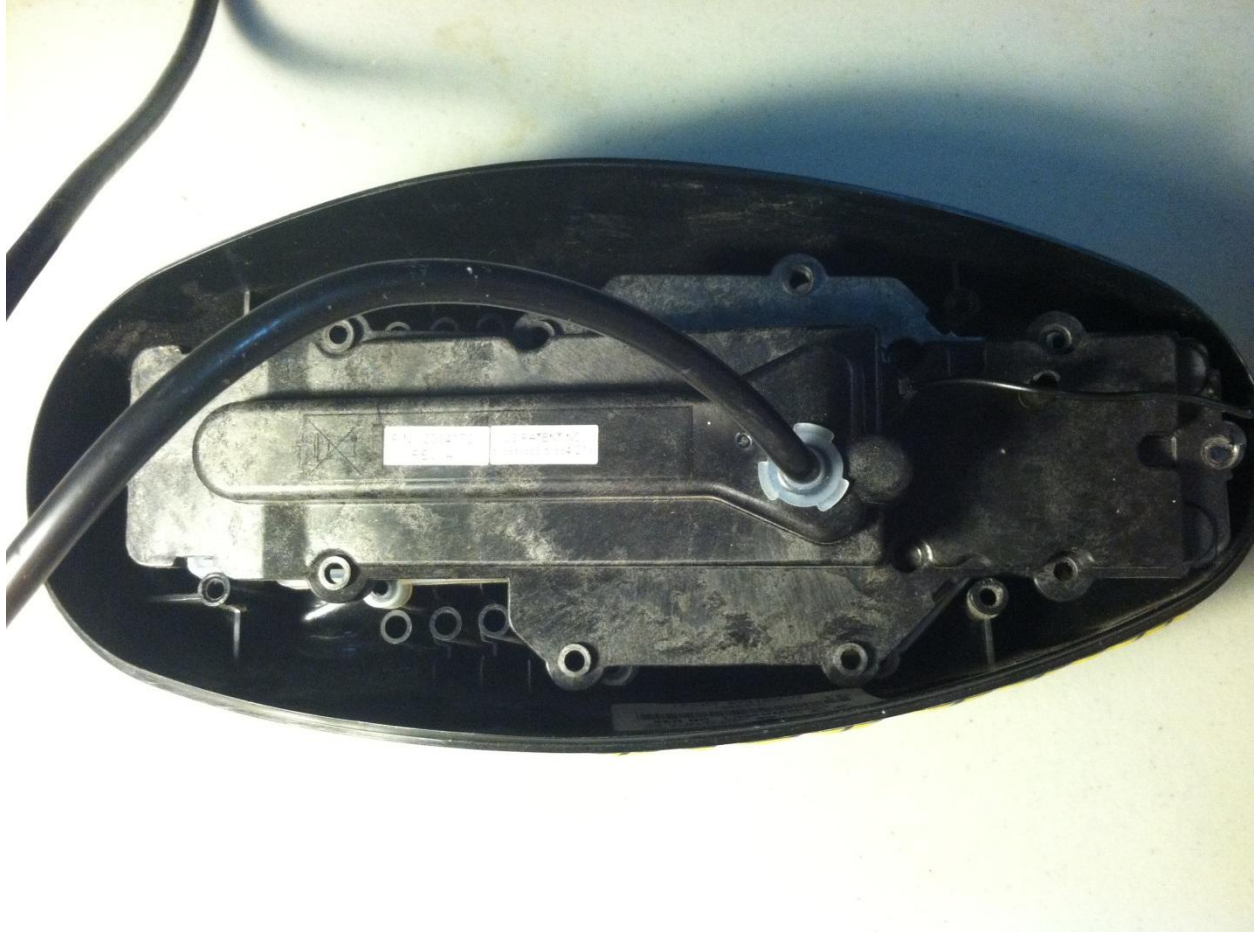
Figure 1 - Underside of motor controller assembly. Antenna is the black wire on the right side of the photo Approx. 3 in. long.
