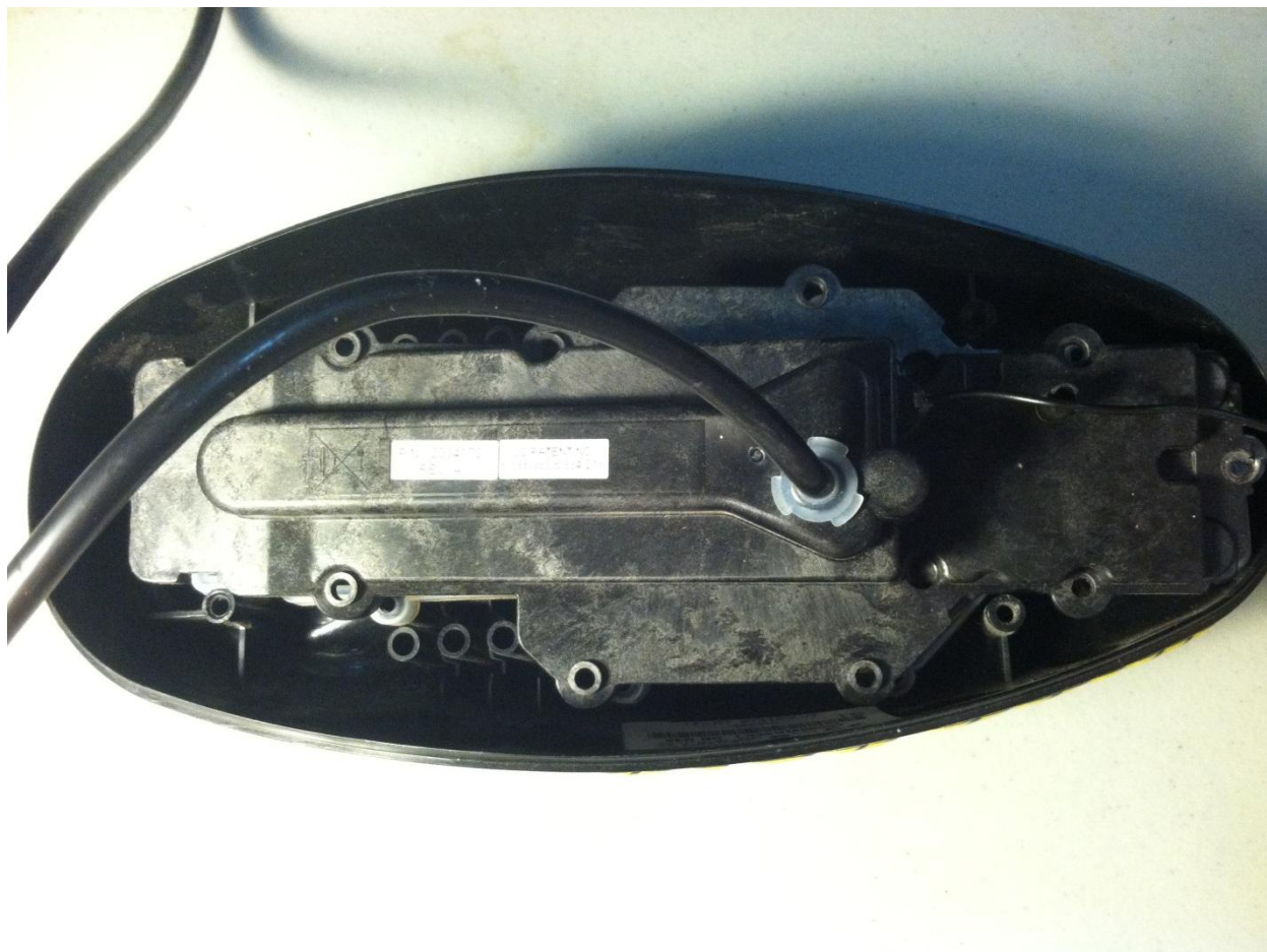
Figure 1 - Bottom of motor controller assembly
