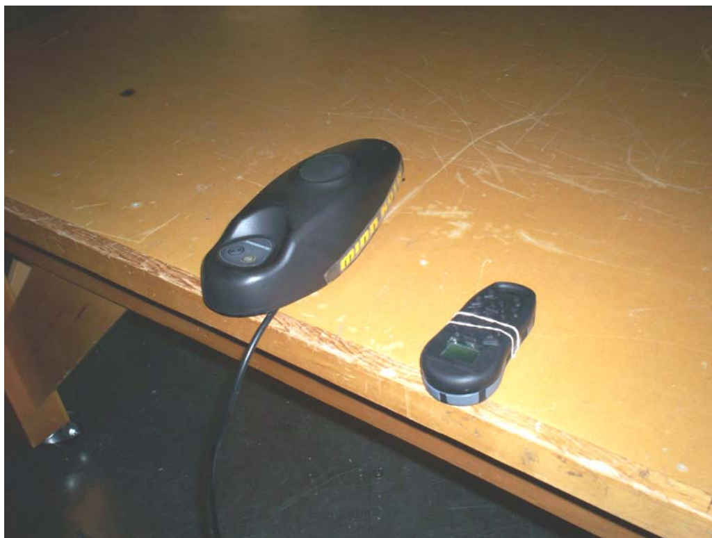
Figure 4 - Radiated Emission Test Setup, 30MHz - 1GHz, with i-Pilot Remote
