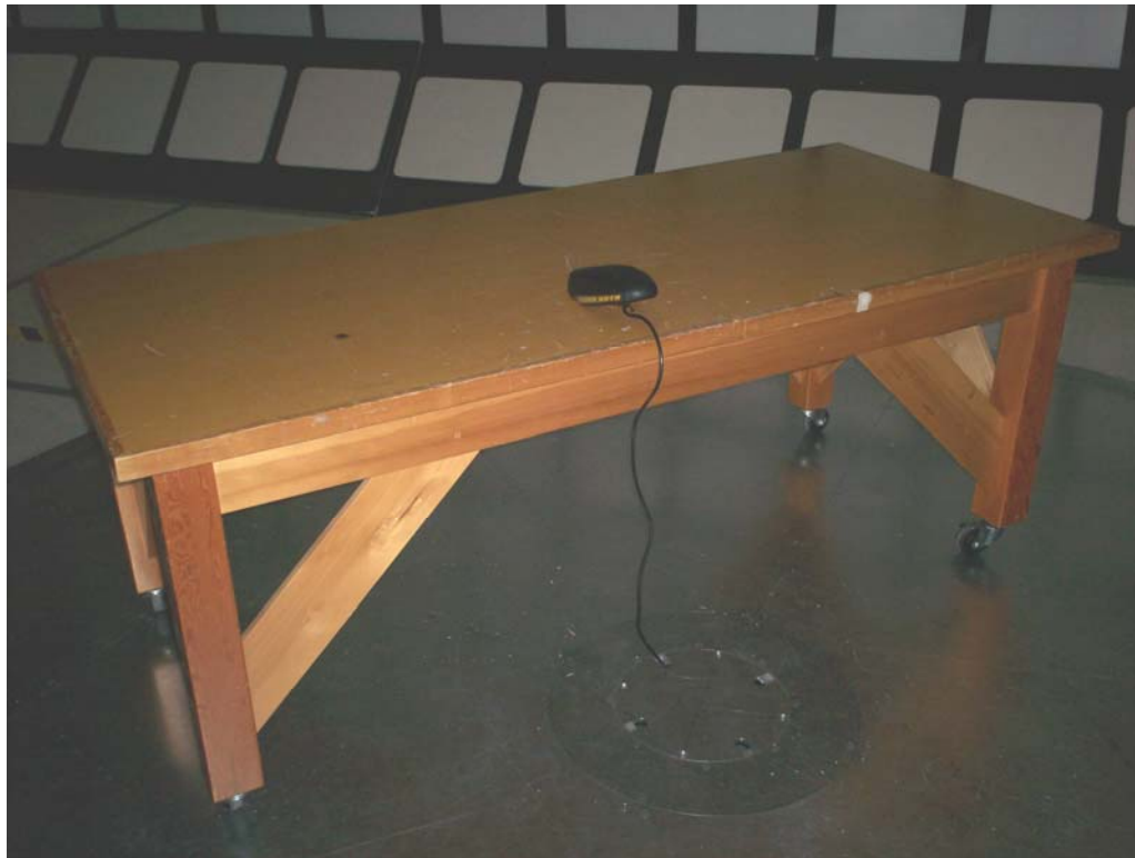
Figure 1 - Radiated Emission Test Setup, 1GHz - 25GHz
