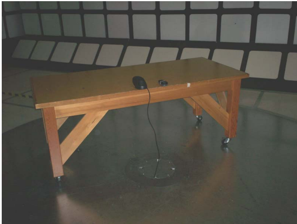
Figure 3 - Radiated Emission Test Setup, 30MHz - 1GHz, with i-Pilot Remote
