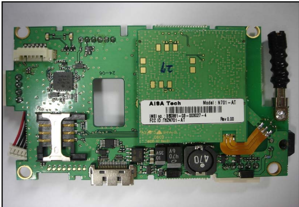
Front View (Quad band GSM/GPRS Module with emulation board)
