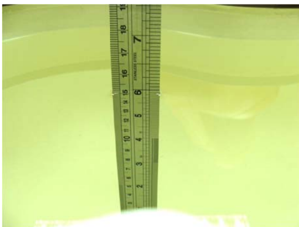
Fig 6.1 Photo of Liquid Height for Head SAR
