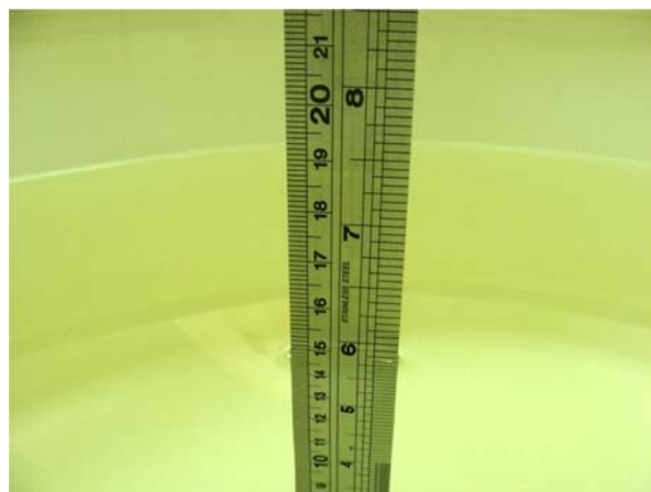
Fig 6.2 Photo of Liquid Height for Body SAR
