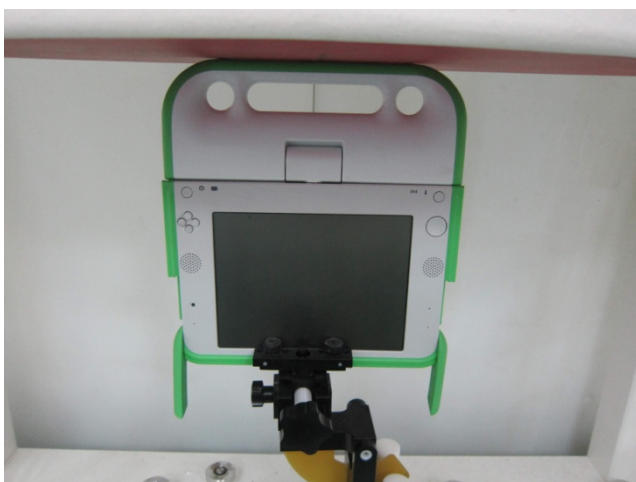
Primary Landscape – Antenna Position 180°
