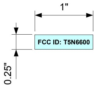
This label will be placed on the bottom side of the Model 6600 roof fan. This will make it visible for the floor. The FCC ID is 8pt
