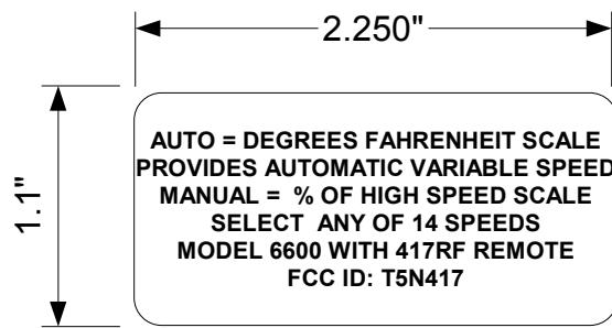
This label will be placed on the bottom side of the Model 6600\_MC417RF remote. This will make it visible for the floor. The FCC ID is 8pt
