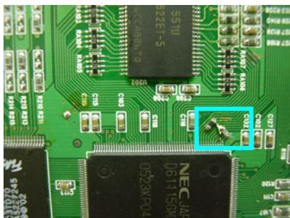
220Ω and 10pF capacitor are inserted additionally in main board.
