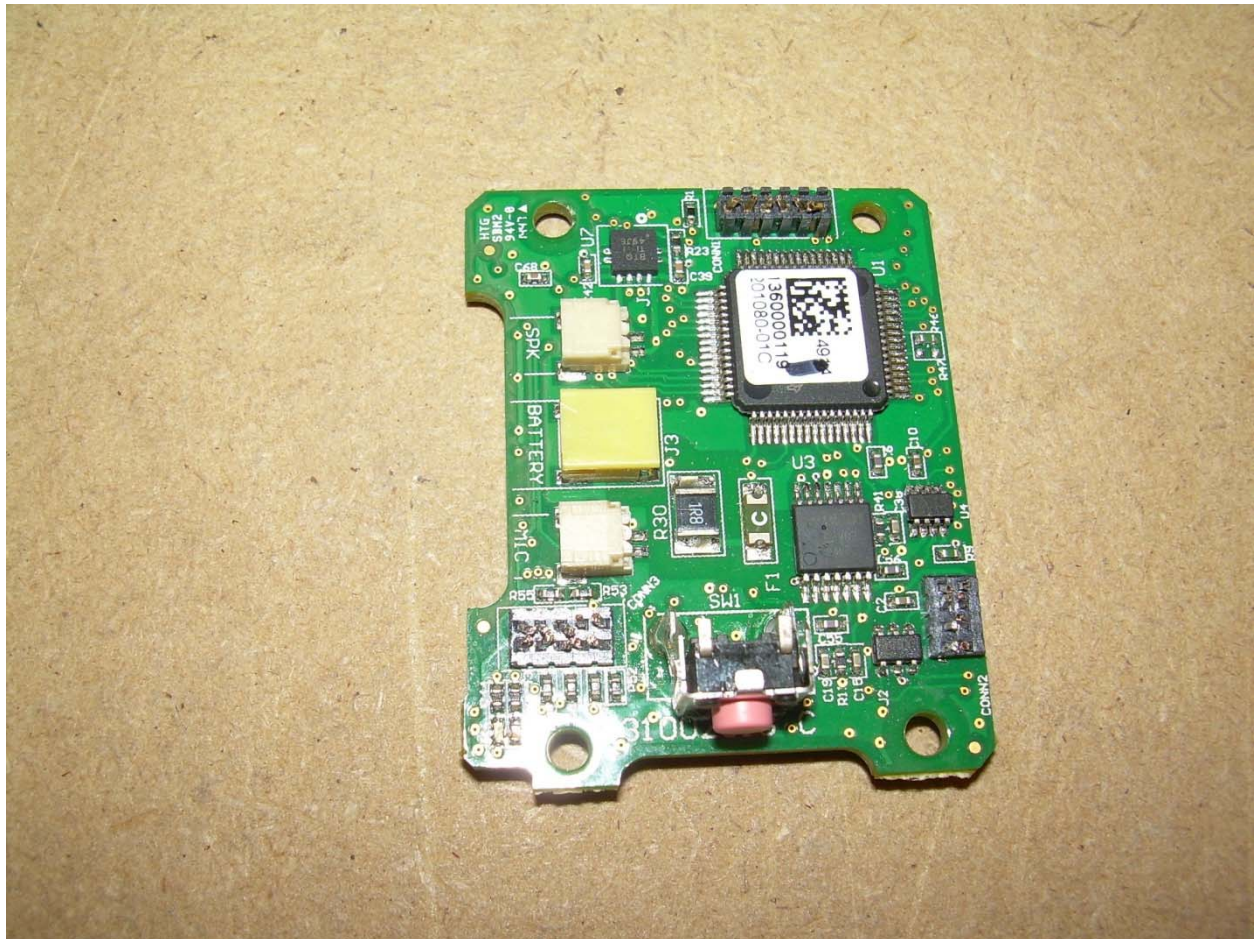
Photograph 12 – Top View of the Audio PCB
