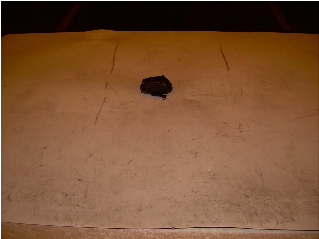
Photograph 4 – Radiated Spurious Emission Test Setup – Horizontal Placement
