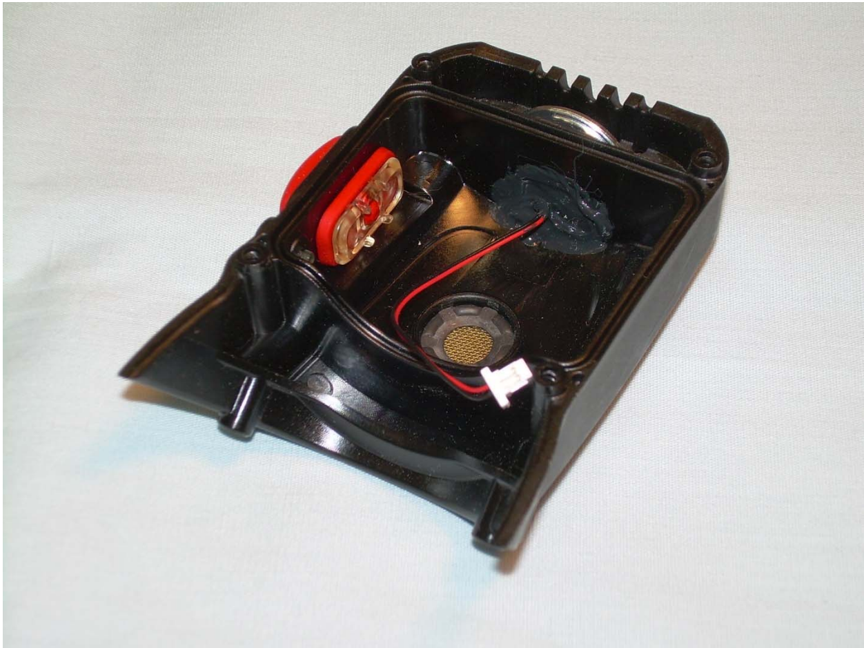
Photograph 9 – View of the Housing with Microphone and Speaker
