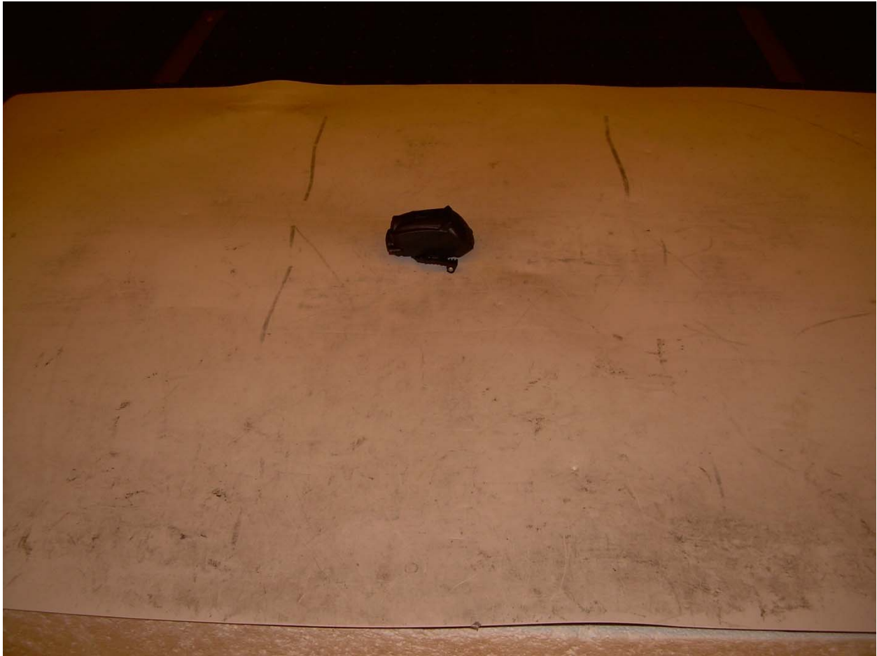
Photograph 4 – Radiated Spurious Emission Test Setup – Horizontal Placement
