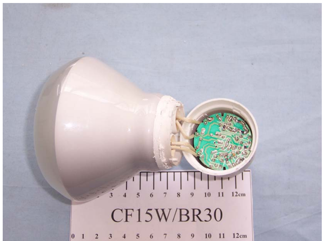
FIGURE 6 COMPACT FLUORESCENT LAMP (M/N: CF 15W/BR30) COVER REMOVED
