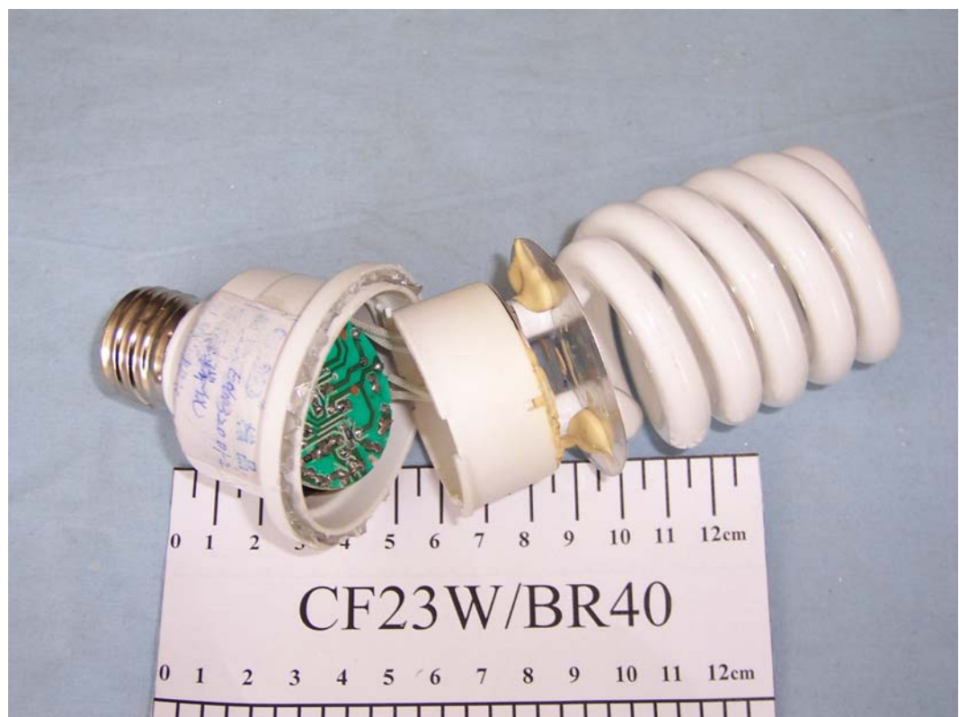
FIGURE 18 COMPACT FLUORESCENT LAMP (M/N: CF 23W/BR40) COVER REMOVED
