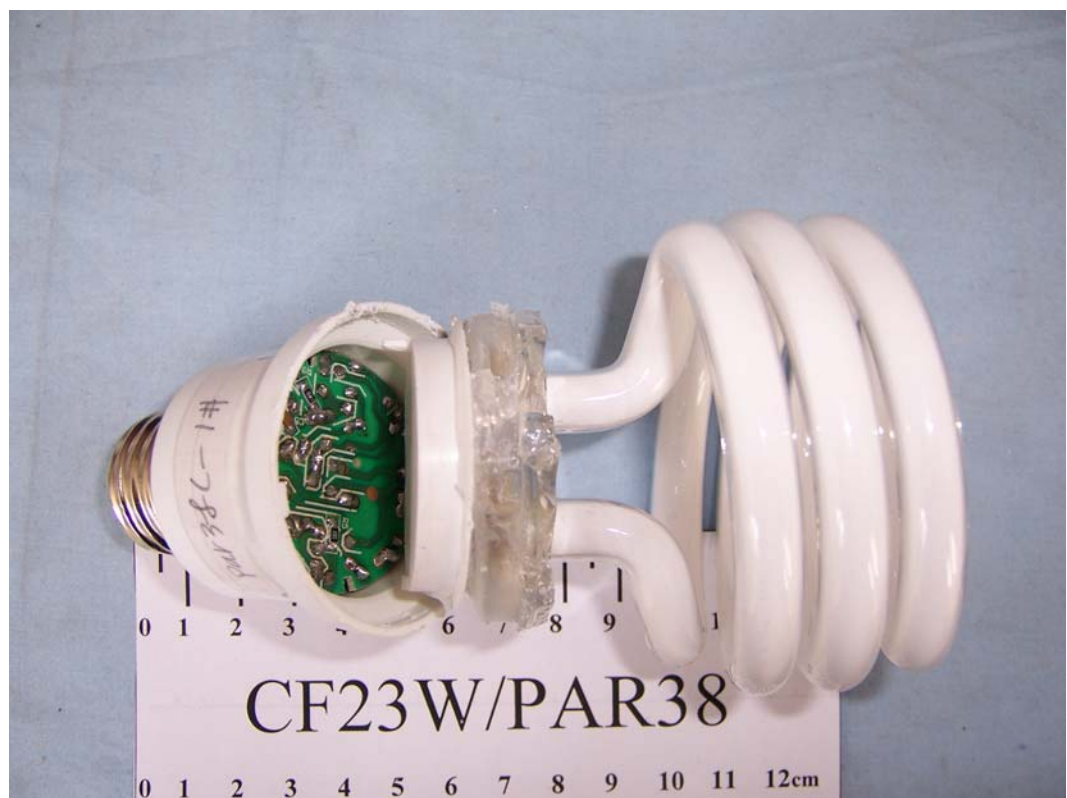
FIGURE 14 COMPACT FLUORESCENT LAMP (M/N: CF 23W/PAR38) COVER REMOVED
