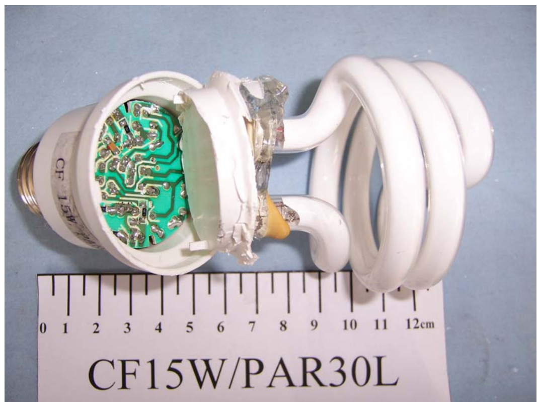
FIGURE 2 COMPACT FLUORESCENT LAMP (M/N: CF 15W/PAR30L) COVER REMOVED
