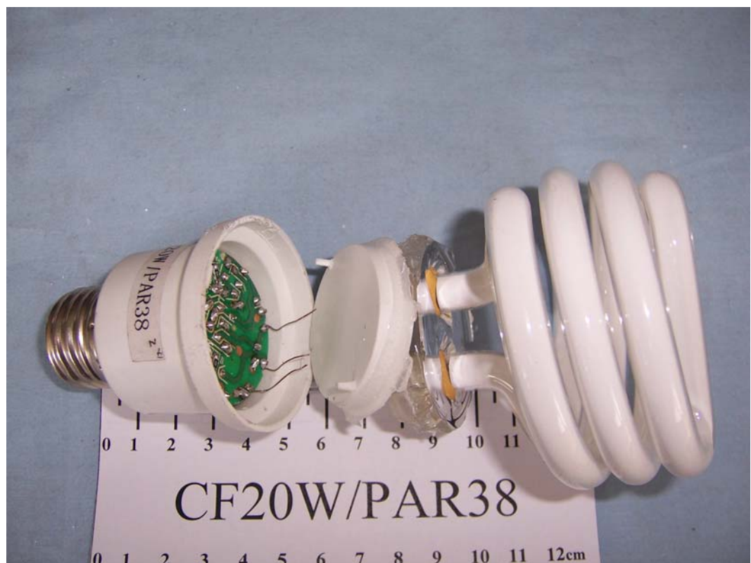
FIGURE 10 COMPACT FLUORESCENT LAMP (M/N: CF 20W/PAR38) COVER REMOVED
