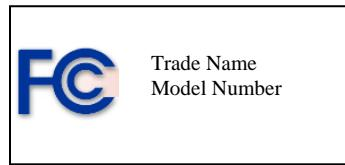
Specifications: Text is black or white in color and is left justified. Labels are silk-screened and shall be "permanently affixed" at a conspicuous location on the EUT.
