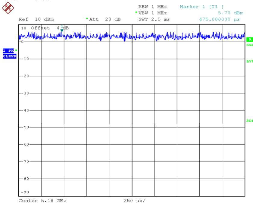
Note: The EUT was programmed to be in continuously transmitting mode and the transmit duty cycle is not less than 98 %, so, the output power and power density should be calculated as Output Power = Measured power + Duty factor
