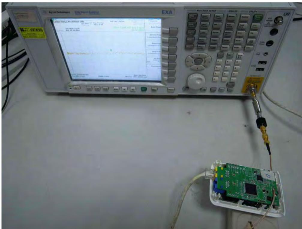
**CONDUCTED EMISSION SETUP**
