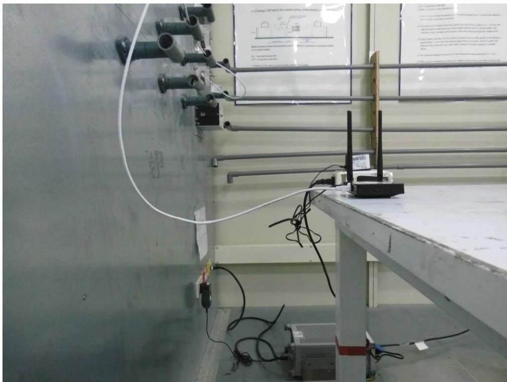
**Radiated Emissions Test Photos****9 kHz to 30 MHz**
