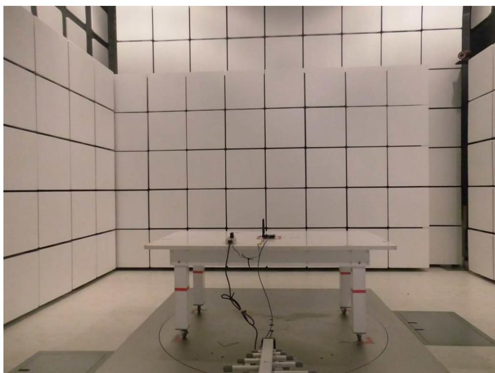
**Radiated Emissions Test Photos****Above 1000 MHz**
